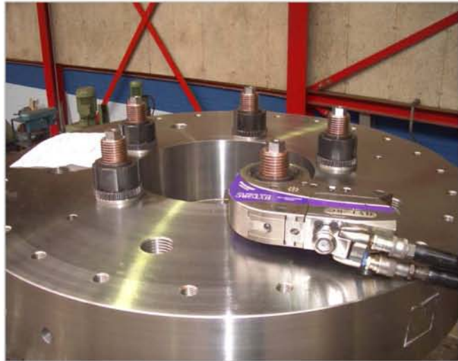
STEALTH ::: conventional bolting procedures, without support and with DISC™ und CLAMP™
