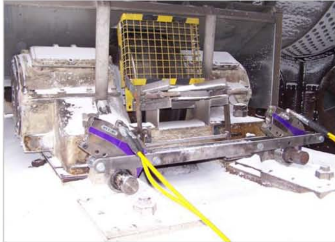
ST-14 TwinTorc - bolt attachment without support arm
